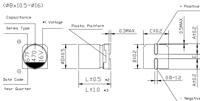
\*1 Voltage mark [6V] represents 6.3V for  $\Phi 4 \sim \Phi 10$ ; \*2  $[L \pm 0.5]$  is applicable to  $\Phi 8 \times 10.5 \sim \Phi 10$ ; \*3  $[L \pm 1.0]$  is applicable to  $\Phi 12.5 \sim \Phi 16$ .Re: Date code and series type — 1<sup>st</sup> digit for Year; 2<sup>nd</sup> digit for Quarter, 4 quarter codes in one year are 1, 4, 7, O; 3<sup>rd</sup> character for Series; FZ Series = F.
